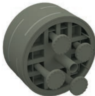
Figure 10 Water injection filters on the outer surface of the steel cylinder (light grey areas)
