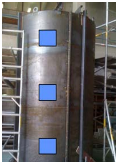
Figure 28 Half-scale test set-up showing three windows to provide access for DIC measurements while the mould is in place
