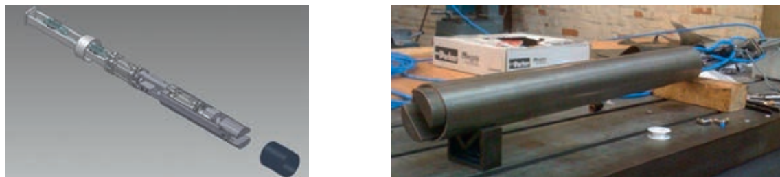
Figure 19 - (Left) 3D design model and (right) prototype of new seismic hammer designed to enhance the generation of S-waves
