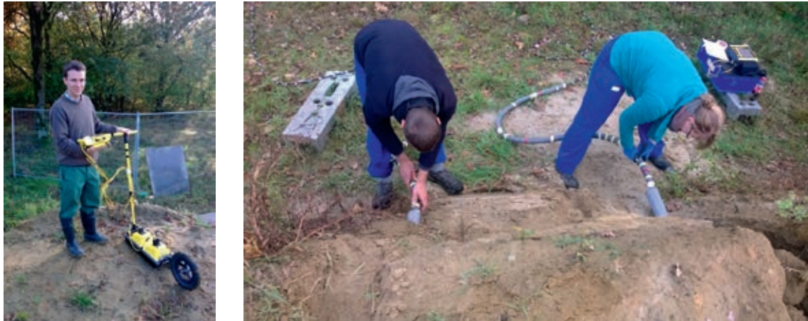
Figure 57 - (left) GPR 500 MHz antenna; (right) pushing source and receiver into the borehole to measure a horizontal plane
