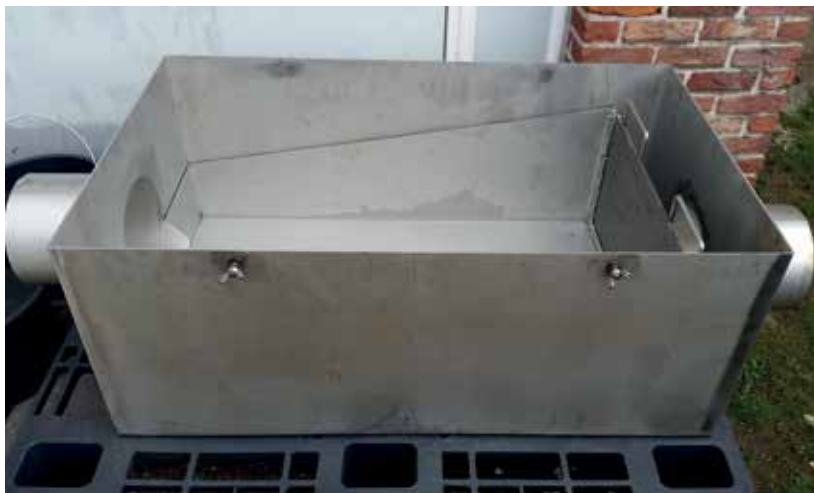
Figure 34 - Prototype of the sediment trap
