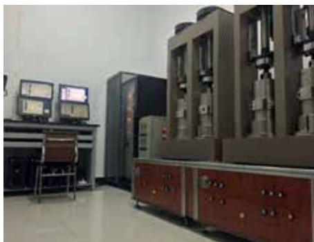
Figure 29 - New THM-coupled triaxial test machine for investigating short- and long-term THM behaviour (IRSM, China)
