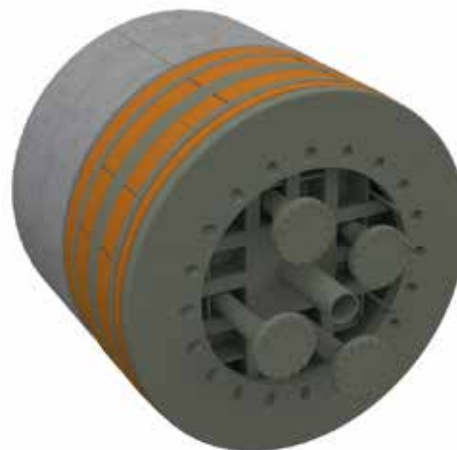
Figure 5 - 3D view of the seal with a central steel cylinder and an annular ring of bentonite (orange) against the clay
