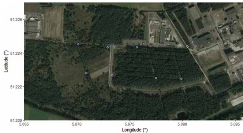
Figure 32 - Location of the nine piezometers used for point dilution tests, part of the additional experimental programme for validation of the hydrogeological models
