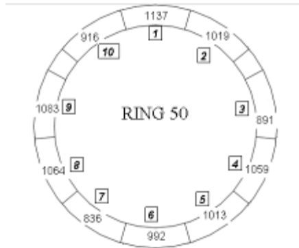
Figure 8.27 : Configuration of ring 50 (segment identities and sequence numbers)
