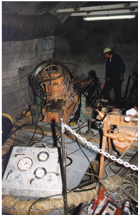
Figure 2.2 : The hydrofracturing test
