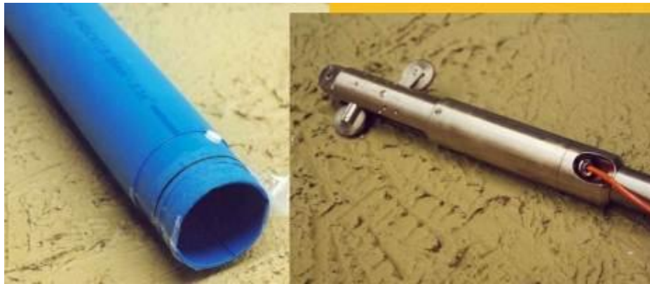
Figure 5.8: Inclinator casing and sensor
