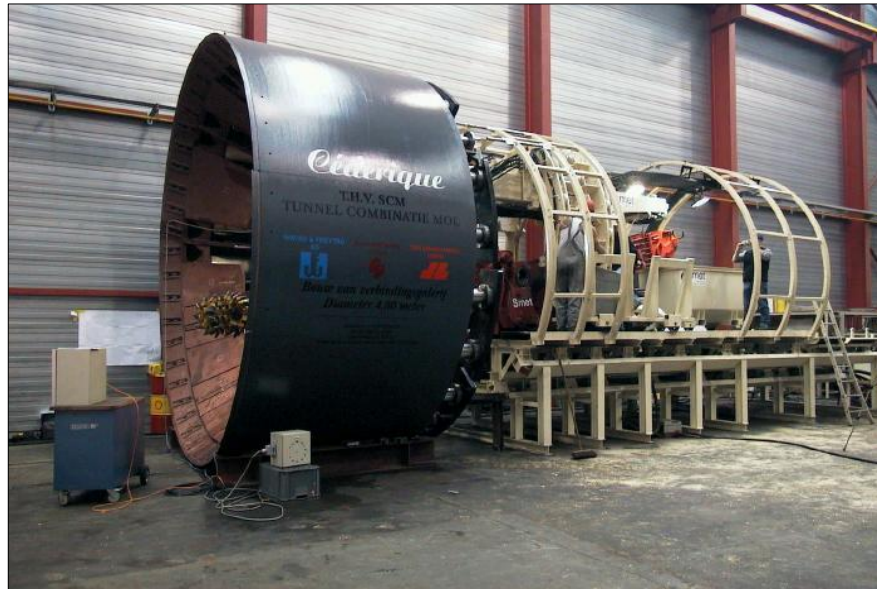
Figure 7.6: Global view of the TBM machine
