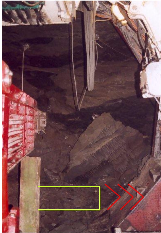
Figure 7.7: Typical fracturation scheme observed at the excavated front
