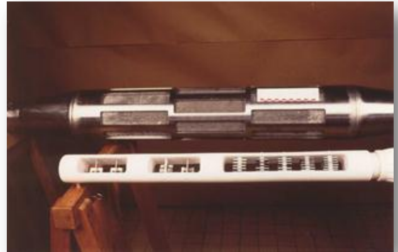
view of a type III corrosion test tube (outer porous concrete tube + inner support tube)
