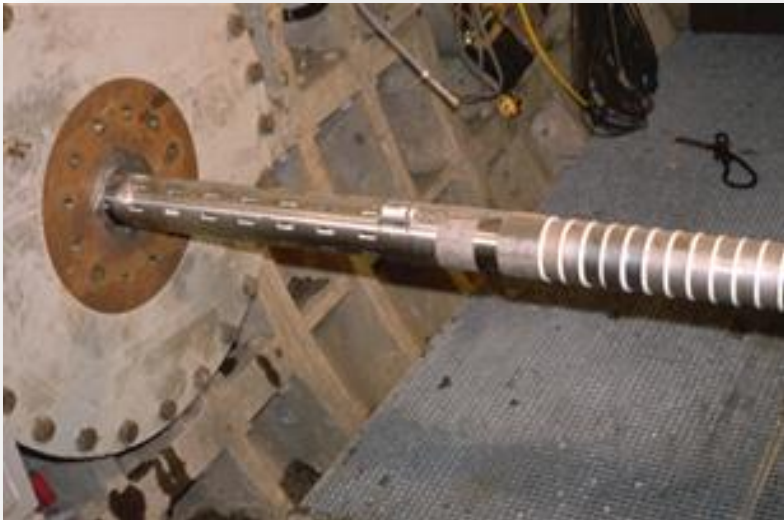
view of a type I corrosion test tube during installation in the underground research facility
