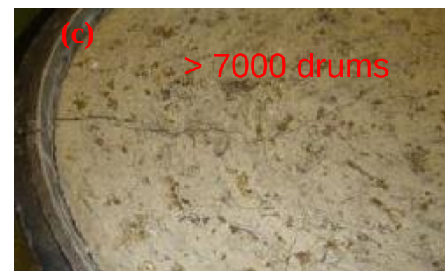
ASR at containment building of Tihange NPP (a) [FANC 2013], Seabrook NPP (b) [Saouma et al. 2014] and cemented waste drum from Doel NPP (c) [FANC 2014]
