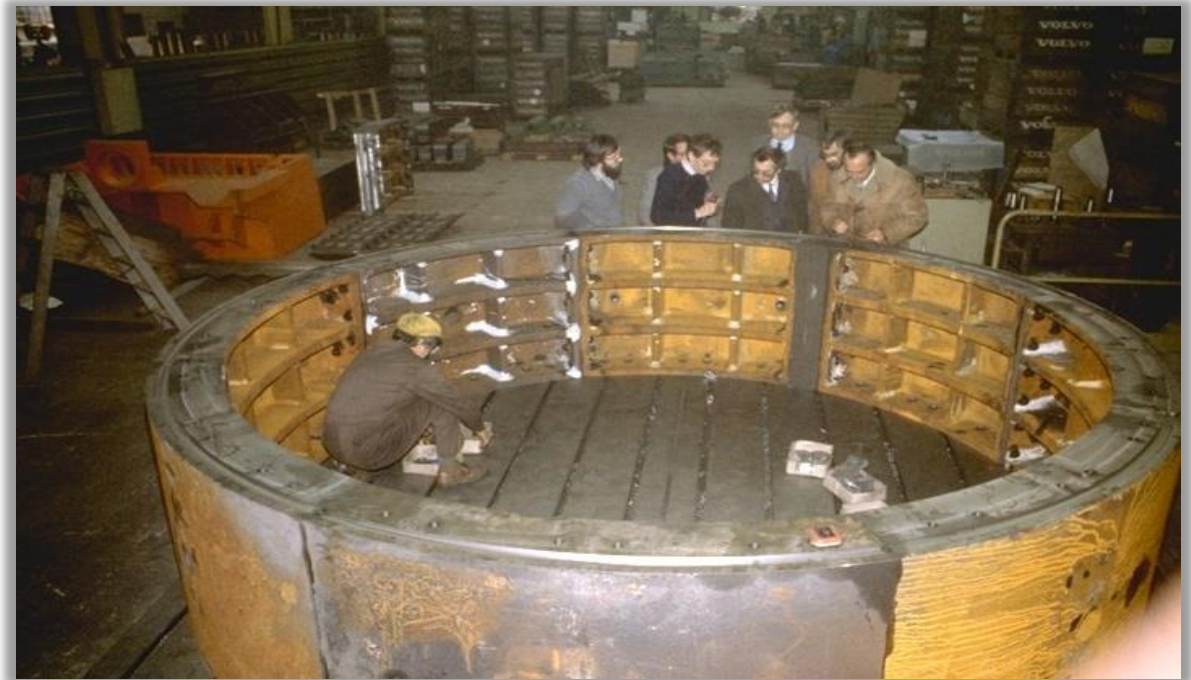
Prefabricated cast iron lining
