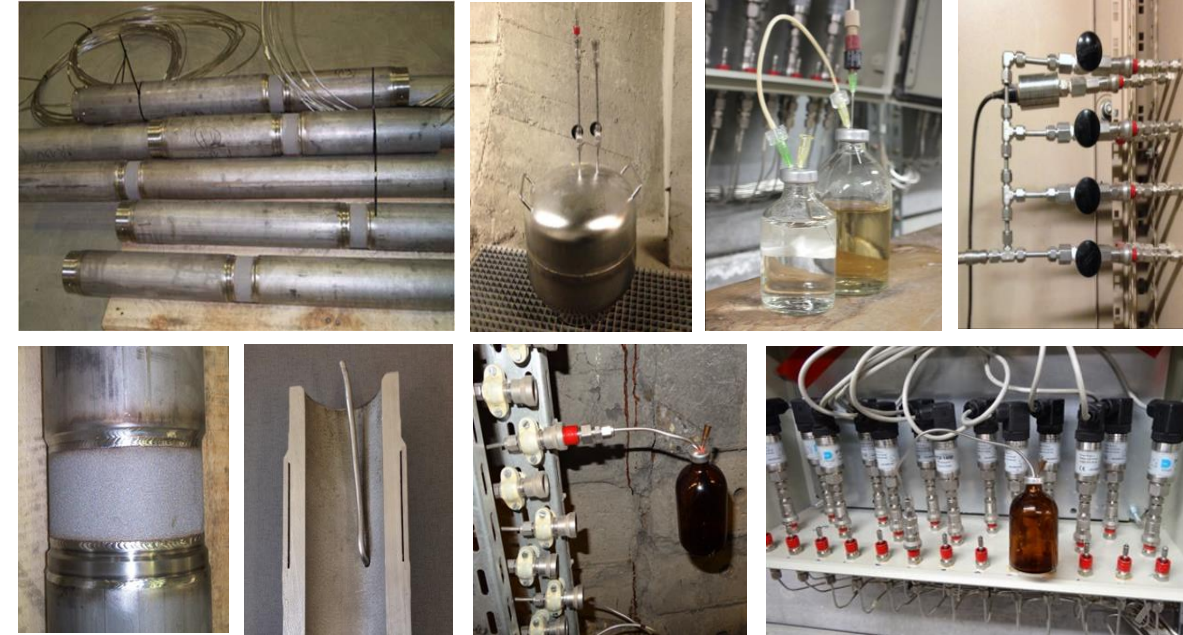
In situ - piezometers
