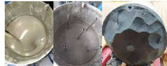
Figure 1 Geopolymer composition during mixing (left), after curing (middle) and cut bottom of the drum after curing (right)
