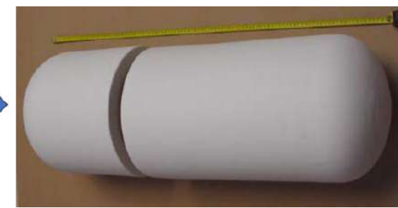
Andra's half-scale model of \text{Al}_2\text{O}_3/\text{SiO}_2 VHLW container
