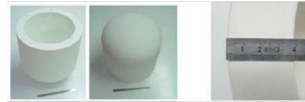
Andra's half-scale model of \text{Al}_2\text{O}_3/\text{SiO}_2 VHLW container
