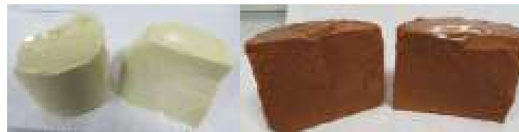
50 vol% loading of Nevastane EP 100 in MetaMax geopolymer (left) and Argicem geopolymer (right).
