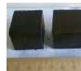
Geopolymer samples (curing 24h): comp. No.5 (left), and the same with pump oil content of 30 %wt (comp. No.8) of pump oil (right).
