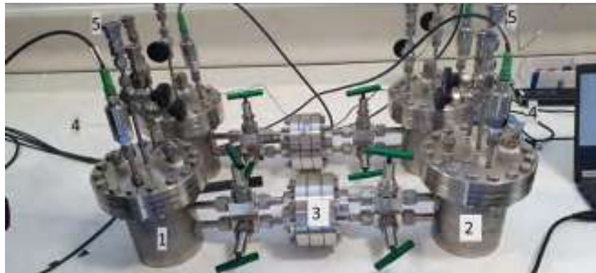
Double-through diffusion experiment setup for unsaturated clay (SCK CEN)
